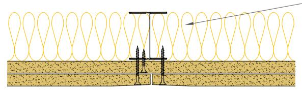
SPEEDLINE 50mm 'I' Studs at 600mm Ctrs
